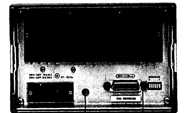
Opening for bringing out sinewave or squarewave output IEC-bus connector and address switch
